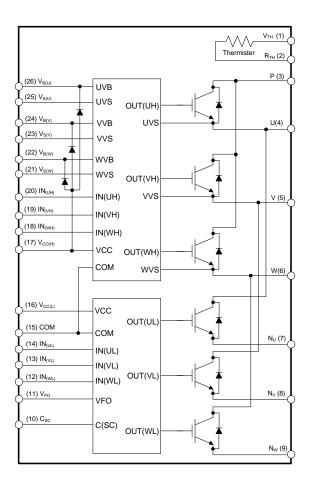
Figure 3. Internal Block Diagram
