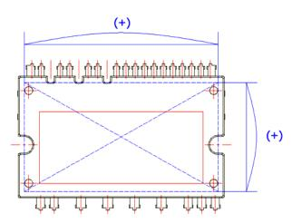
Figure 9. Flatness Measurement Position
