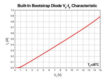
Figure 7. Built-In Bootstrap Diode Characteristic
