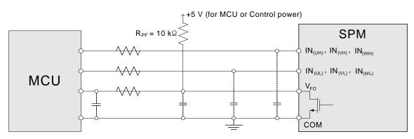
Figure 14. Recommended MCU I/O Interface Circuit
