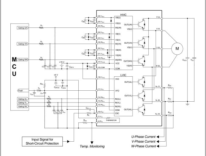
**Figure 15. Typical Application Circuit**
