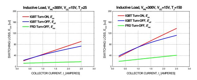
Figure 5. Switching Loss Characteristics (Typical)
